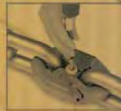
Assembly of a RUD flat connector
